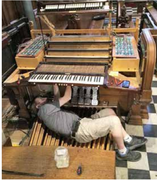
The 1926 Casavant pipe organ is being modernized with solid state components replacing aging leather contacts and digital technology adding to its tonal resources.
